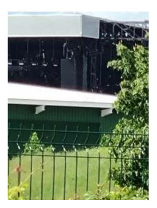
A favourite 'how not to' event from 2022. This was the Killers at Doncaster Keepmoat Eco-Power Stadium. More than half the line array system and all of the flown bass cabinets were rigged above the height of the stadium roof. Noise levels at a hotel 400m from the audio system were 95dBA with sub-bass shaking the building. Click the video (right) to hear the impact.
